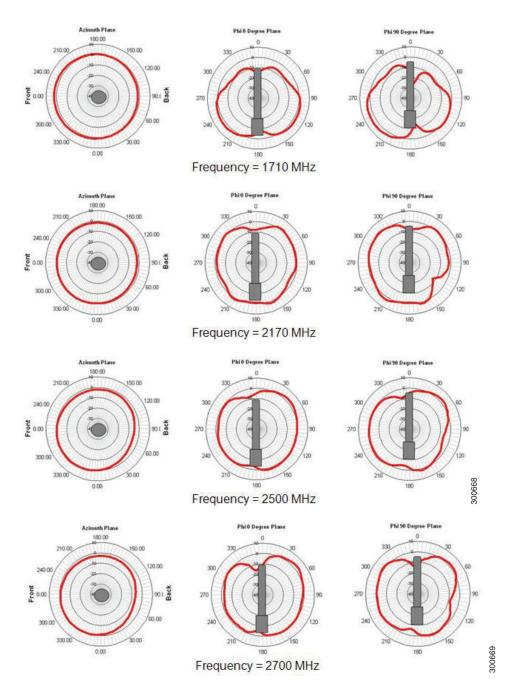
Figure 4-3 Outdoor Omnidirectional Antenna Radiation Patterns (2 of 2)
