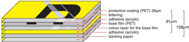
Brother P-touch laminated TZ tapes consist of six layers of materials, resulting in a thin, extremely strong label. Characters are formed with a thermal transfer ink and sandwiched between two protective layers of PET (polyester film). The result is a virtually indestructible label that can withstand even the harshest conditions.
